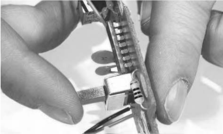
Figure 12.8 Finding the clock resistor (finger on right).
