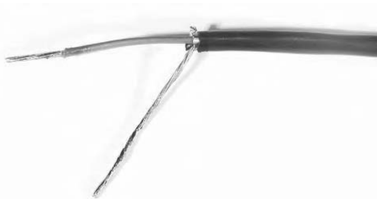
Figure 7.2 Shielded cable prepared for soldering.
