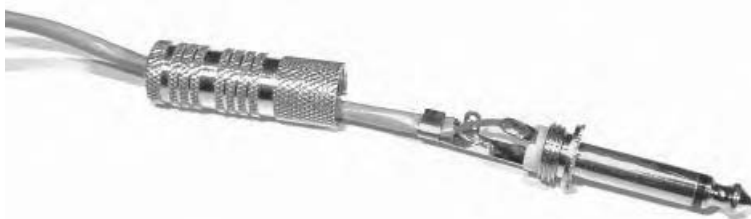
Figure 7.4 Cable soldered to plug.
