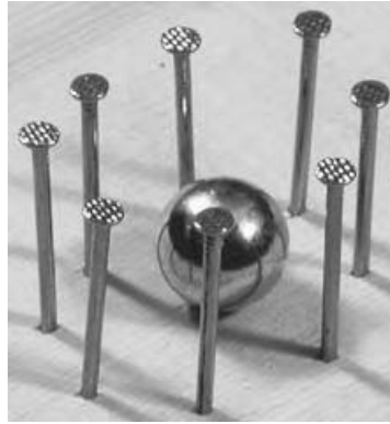
Figure 16.5 A homemade tilt switch.
