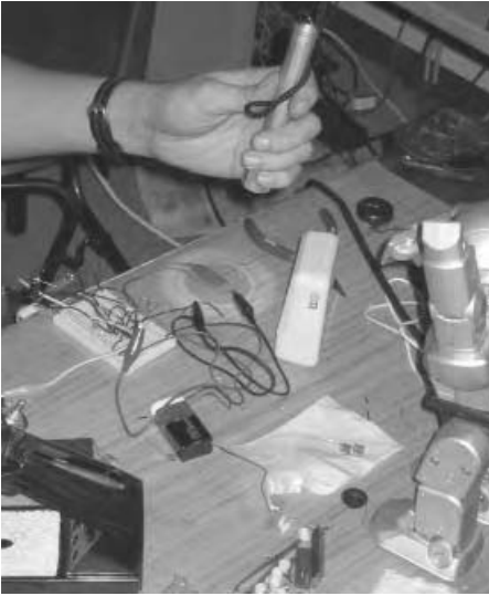
Figure 18.11 Playing a photoresistor-controlled oscillator with a flashlight.
