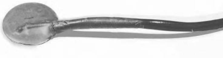
Figure 7.5 Contact mike encased in Plasti-Dip.
