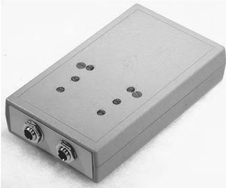
Figure 19.6 A boxed photoresistor-controlled Hex Oscillator.
