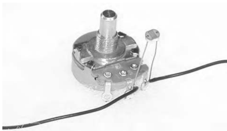
Figure 15.5 A potentiometer and photoresistor in parallel.
