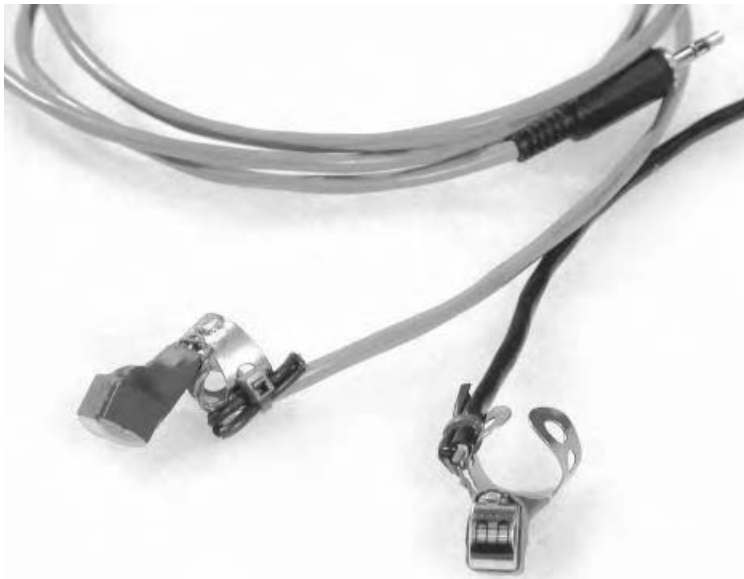
Figure 9.3 Tape heads mounted on fingerpicks, Nicolas Collins.
